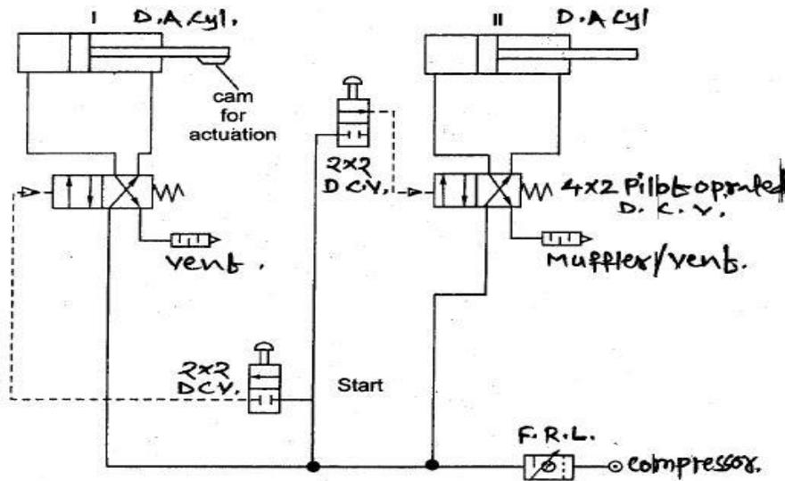
fig. Position based sequencing
